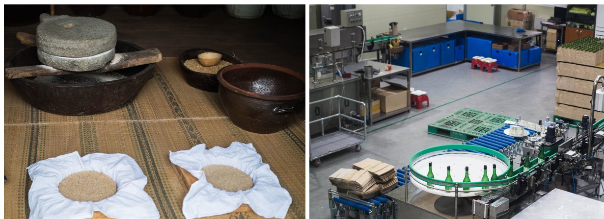
Fig. 13: (Left) Nuruk and various traditional soju-making apparatuses on display at the Pak Chaesŏ Andong Soju Factory. While these apparatuses are on display, the actual product is made using a “modern” production process using jacketed fermenters, a portion of which is shown on the right. The soju is still advertised and marketed as a “traditional” Andong soju. Courtesy of Joon Kim.
